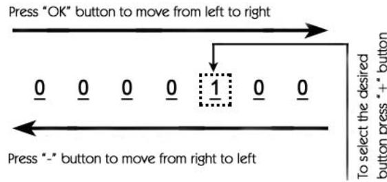
To access the available menu it is necessary to press “+” and “OK” buttons at the same time. The frame below will be displayed:
