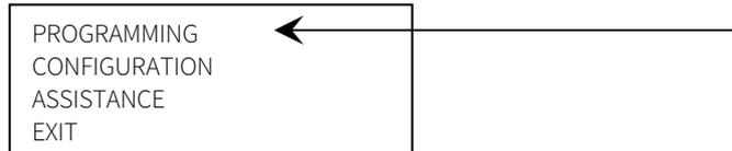
From the Programming Menu it is possible to set or change the machine operating parameters. Here below are listed and described the programmable functions in the different Programming Menu sections.
