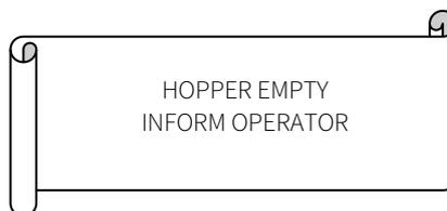
This message means that the change machine finds the coin hopper empty and therefore it cannot make the change operations.
