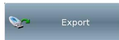
This screen (shown in Figure 111 below) allows to access the data export functions provided by the system. Make sure you plugged a FAT32-formatted pen drive into the special USB connector inside the machine.
